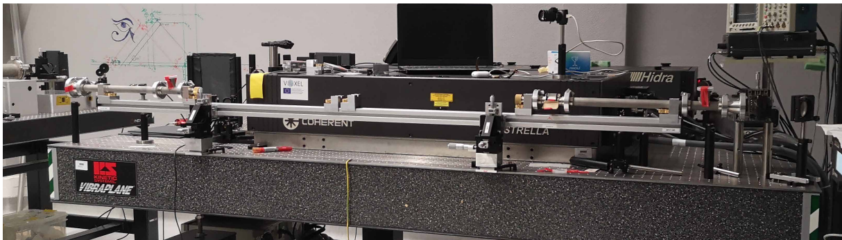
Figure A.3: Installation of the input and output tubes onto the rail.
