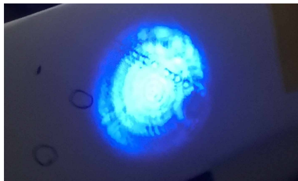
Figure 2.8: Second Harmonic signal through the damaged BBO.
